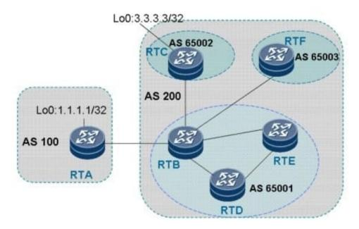
As shown in the figure, RTA belongs to AS 100 and has an EBGP neighbor relationship with RTB. RTB, RTC, RTD, RTE, and RTF belong to AS 200.RTB, RTD, and RTE are assigned to AS65001, RTC to AS65002, and RTF to AS65003.
