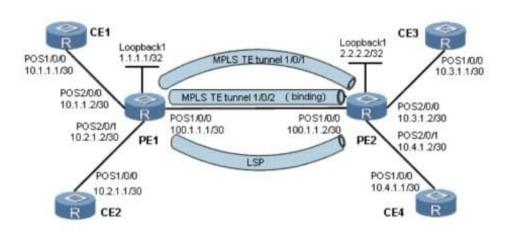
This figure shows the MPLS L3VPN networking. CE 1 and CE 3 belong to VPN A. CE 2 and CE 4 belong to VPN B. Two MPLS TE tunnels (5 Mbit/s and 10 Mbit/s) and an LSP tunnel are set up between PE 1 and PE 2.It is expected that a tunnel policy is configured on PE 1 to distribute traffic in the three tunnels and MPLS TE tunnels are preferred. Configurations on PE
