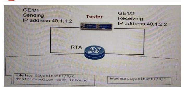
As shown in the figure, complex traffic classification is configured for RTA\\'s upstream GigabitEthernet 1/0/0. The QoS is configured as follows:
