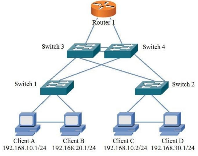
If Client B sends a packet to Client A, what is the highest level of the network hierarchy that the packet will transverse?
