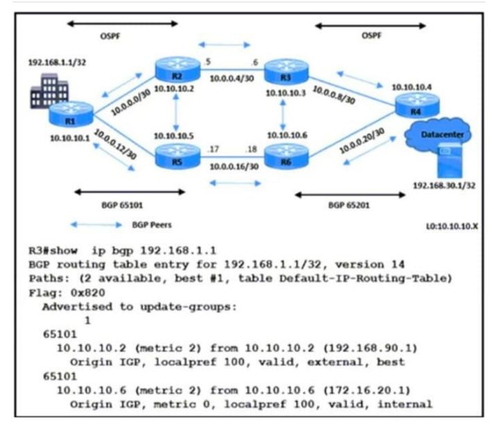
Refer to the exhibit. A network engineer is implementing BGP in AS 65101 and AS 65201 R3 sends data traffic to 192.168.1.1/32 via the path R3-R2-R1. The traffic must travel via alternate path R6-R5 for prefix 192.168.1.1/32. Which action must be taken to meet the requirement?
