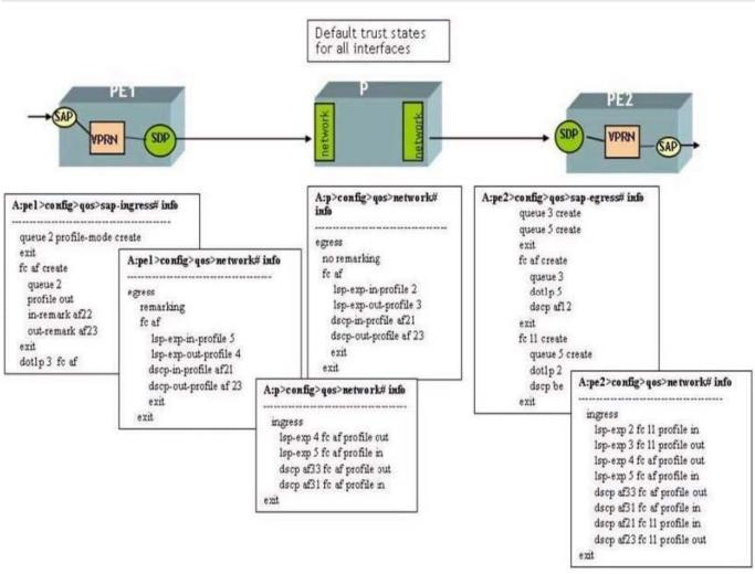
All interfaces are using their default trust states and MPLS is used as the transport tunnel. The SAP-ingress, SAPegress, and network QoS policies have been configured as shown below. Assume that the default network-queue policy is used on each router.
